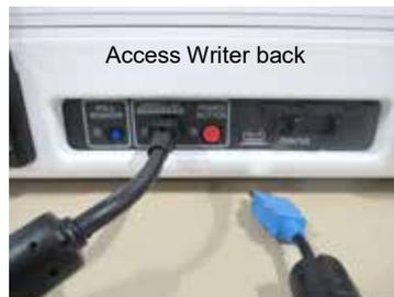
**14.** Connect blue end of USB cable, notched side up, to Access Writer (slide 'Printer' door to right) and black end of cable to Access Ballot Printer.
