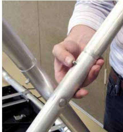
Press metal buttons to attach and lock in place.
