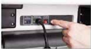
5. Press red POWER button on back of Access Writer to power it down completely
