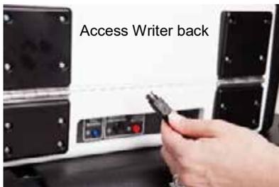
**13.** Remove all cords & cables from Access Station cords bag. Move to the back of Access Writer and attach power cord/power brick, flat side up. Insert firmly. You should hear a small click.
