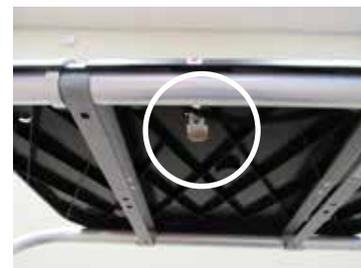
**9.** Push slide underneath surface towards the back to secure Access Writer in place. Pull up on the Access Writer handle to make sure it is secured.
