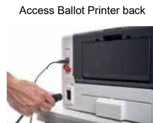
Attach printer power cord to back of printer. Load printer paper.
