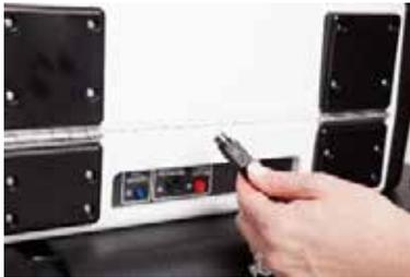
Gently pull back sleeve and unplug Access Writer power cord/brick—pull straight out, do not yank or jerk in different directions. Disconnect Access Writer from printer. Disconnect all other cords & cables from printer. Place cords, cables and surge protector in Access Station cords bag.
